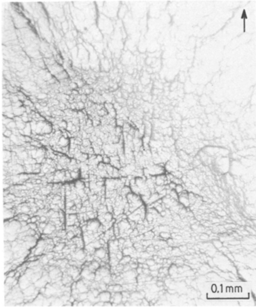
Figure 9 High-magnification photograph of the central region of Fig. 4 after 23 000 impacts showing the network-line structure of the central cracks. The small arrow indicates the extrusion direction.
